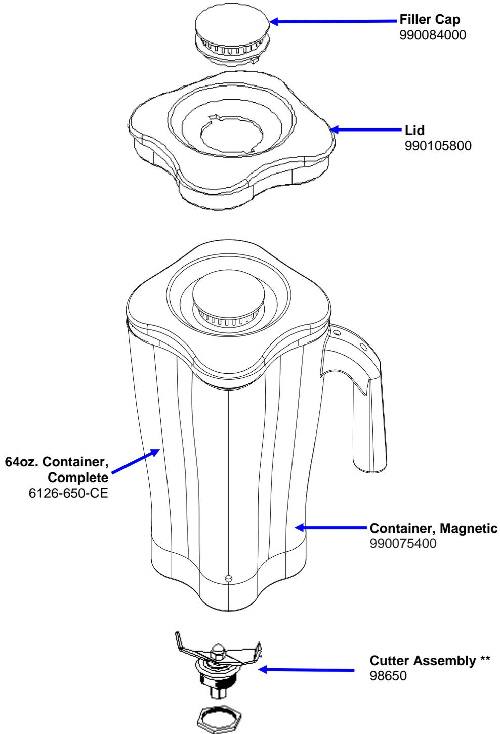
\*\*Cutter Assembly Includes: Blade, Lock Washer, Hex Nut, Drive Coupling Attachment and Cutter Bearing Assembly.
